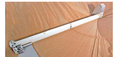
Silo funnel emptying via screw-conveyor
